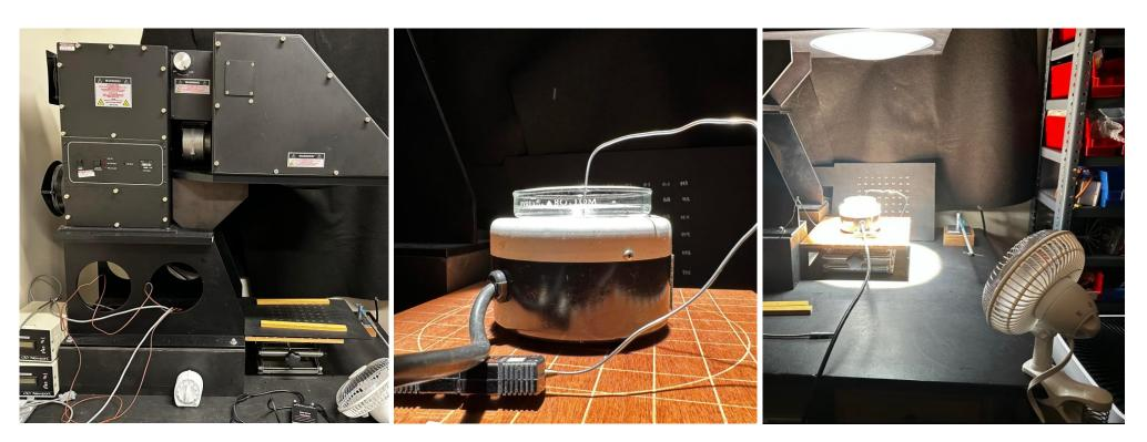
Figure 4. Solar simulator experimental setup with fan for temperature stability
