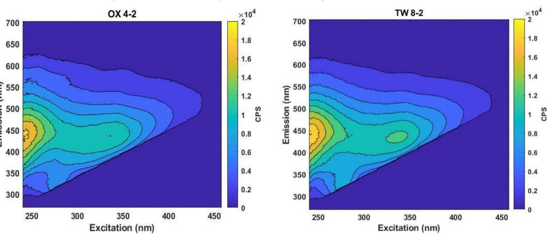
Figure 6. Excitation and emission matrix spectra (EEMs) for Oxidation Ponds (OX 4-2) and Treatment Wetlands (TW 8-2)
