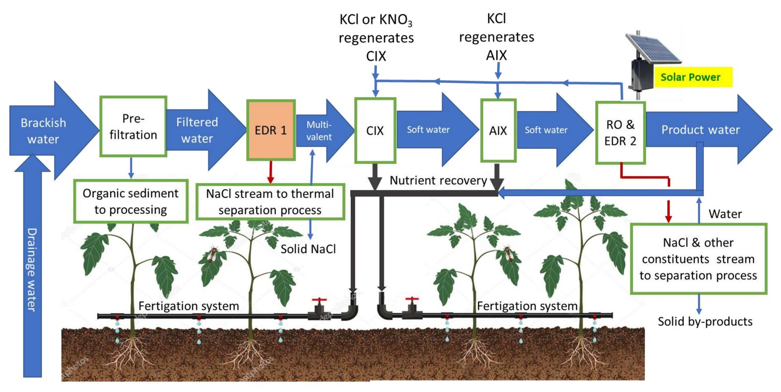
Schematic process flow diagram showing innovative technology for producing irrigation water and nutrients from saline water sources. EDR: Electrodialysis Reversal; CIX: Cation Exchange; Aix: Anion Exchange; RO: Reverse Osmosis.
