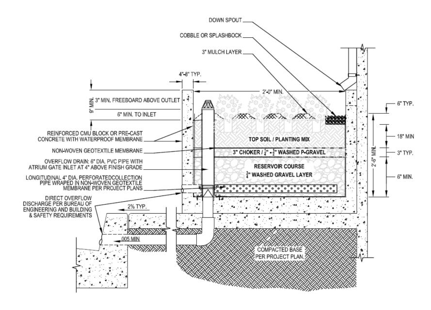
**Figure 3.** Bioretention cell cross section details, City of LA standards (left), field scale cell (CPP systems) (right)
