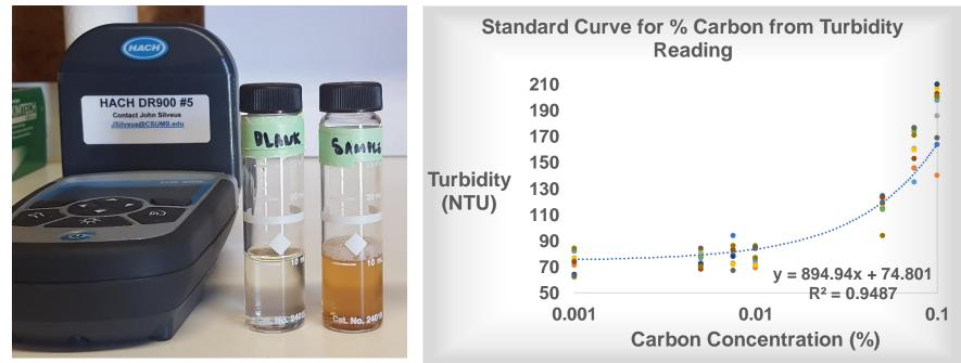
Fig 7. Left: Sample cells used in HACH Colorimeters for NO<sup>3-</sup> readings. **Right:** Standard curve allows carbon concentration to be calculated from turbidity.
