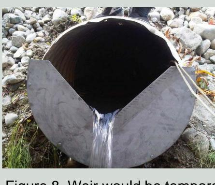
Figure 7. V-Notch weir (USBR,2001)
