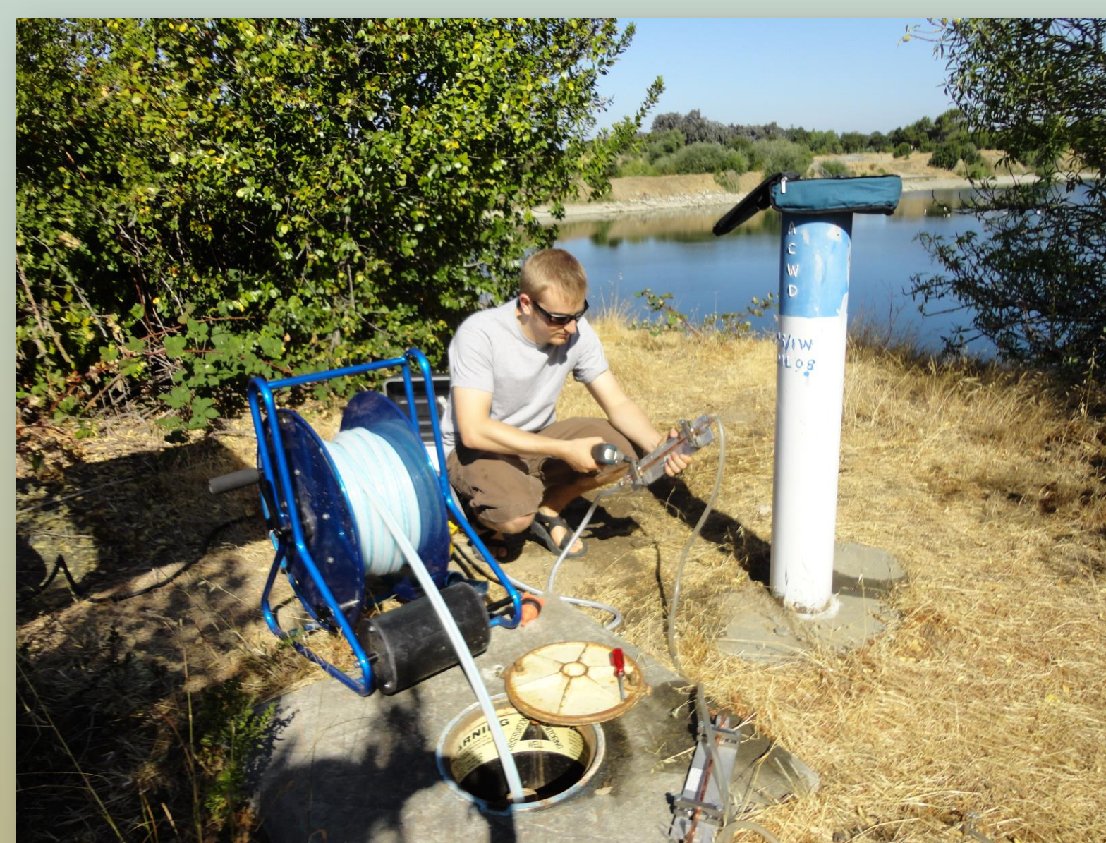
Figure 3: Sampling a monitoring well.
