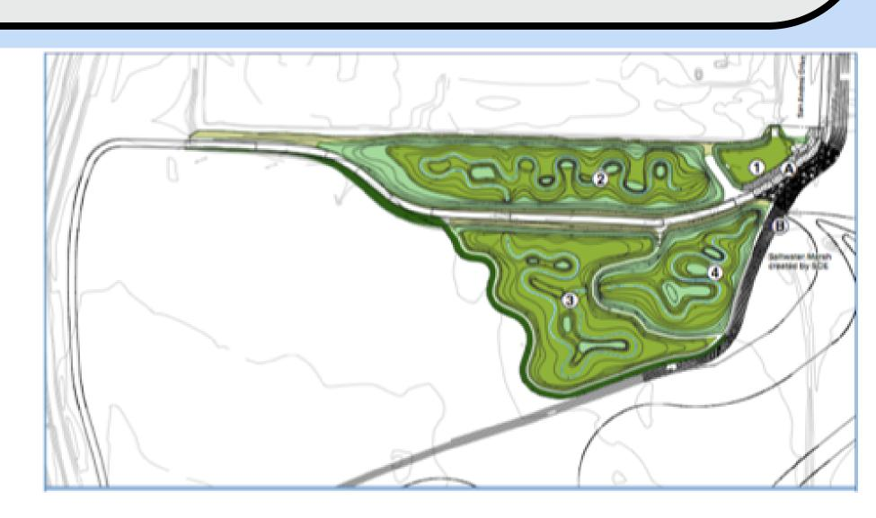
Figure 1. Letter A represents where the urban runoff enters into the treatment pond one. It is then diverted under a constructed berm by a culvert to direct flow into treatment pond two. It is then filtered through and underneath the trail through a culvert into treatment pond three, where it filters through again and under a berm through a culvert into treatment pond four where it is filtered for a fourth time before being released into the salt water marsh, letter B.
