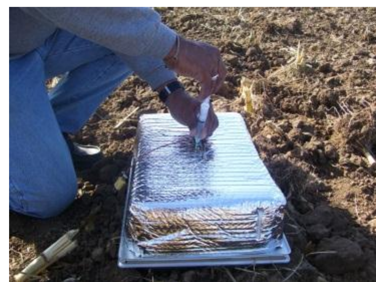
Photos of EPA approved flux chambers techniques being used in the field and the Gas Chromatograph (GC) used for nitrous oxide determinations in the laboratory.
