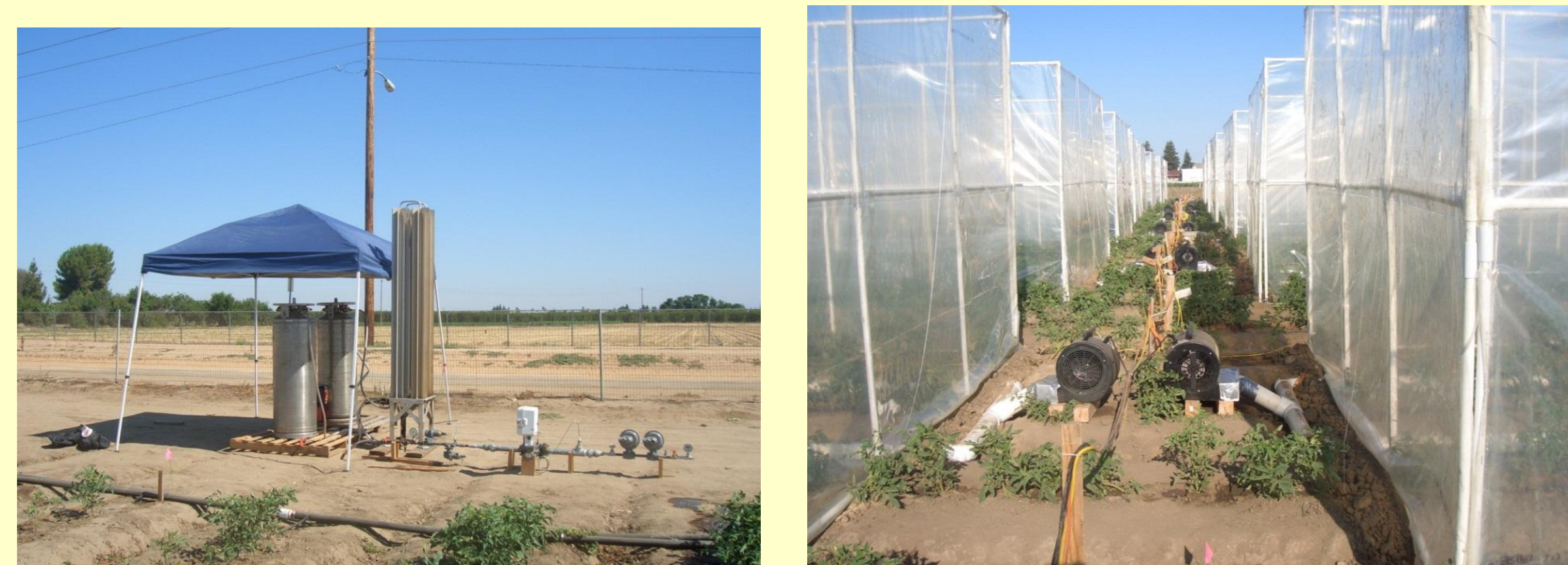
Fig. 1. Open-top chambers with CO 2 delivery system
