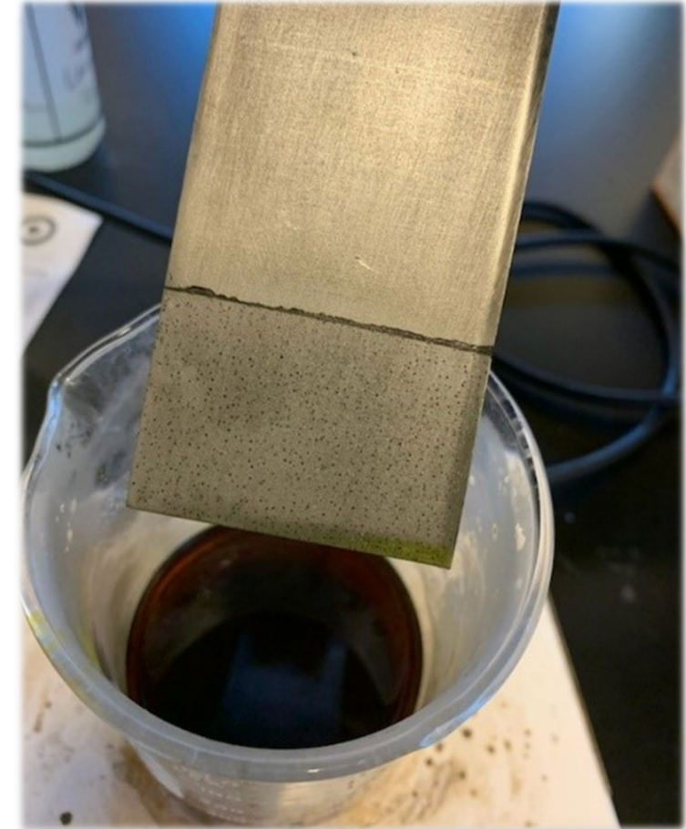
Beaker containing heated ferric chloride and a pitted steel specimen
