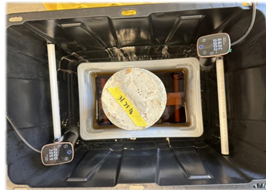
Schematics (left) and an optical image of the experimental setup for the load-coupled corrosion test
