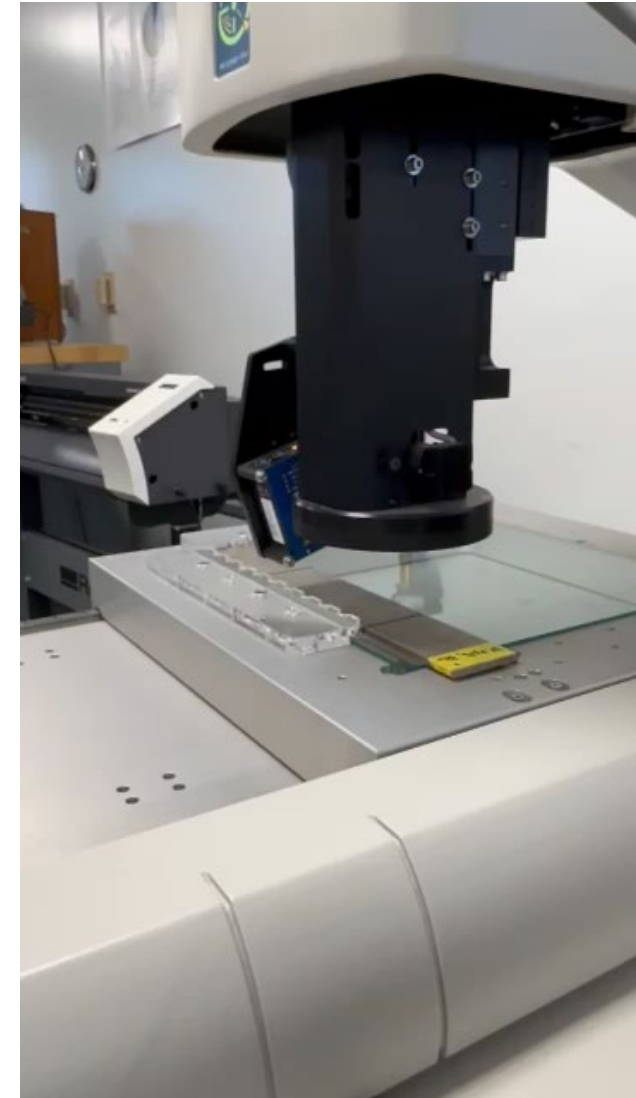
Micro Vu Vertex system with a laser distance scanner during scan of load-coupled specimen
