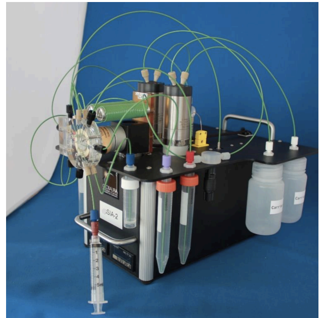
Figure. A miniSIA-2 device used for programmable Flow Injection Analysis.
