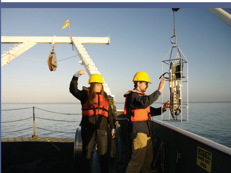
HSU work-study students deploy a CTD from the R/V Coral Sea. Image courtesy of Humboldt State University.
