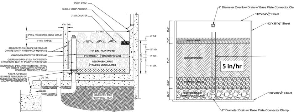
Figure 3. Bioretention cell cross section details, City of LA standards (left), field scale cell (CPP systems) (right)
