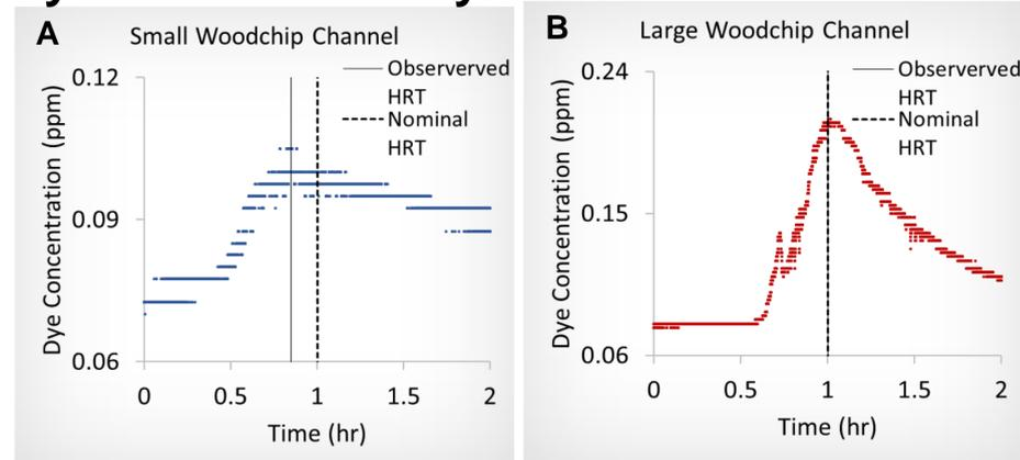
Figure 4: Results of rhodamine dye test indicating observed HRT in (A) small wood chip and (B) large wood chip channels in comparison to theoretical values.
