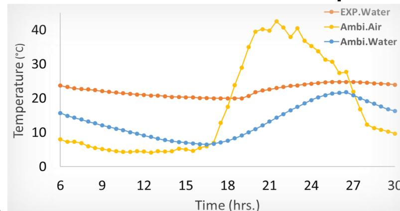
Figure 5: Variations in temperature observed under ambient air, ambient water and experimental conditions.
