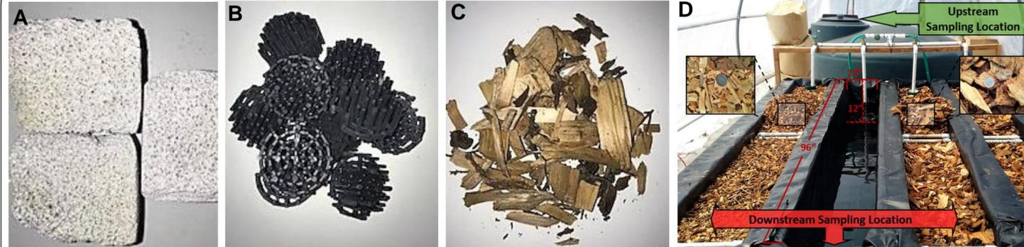
Figure 3: (A) Pumice blocks, (B) plastic bioballs, and (C) pine wood chips used during preliminary research to evaluate viable substrate type for the cultivation of bacteria. (D) Wood chip bioreactor channels separated by substrate grade. The left channel contains small grade wood chips and the two channels on the right contain large grade wood chips.
