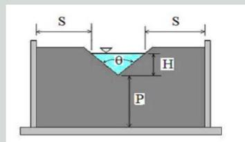
Figure 7. V-Notch weir (USBR, 2001)
