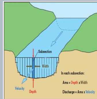
Figure 2. Cross sectional area and flow measurement (Perlman, 2016)
