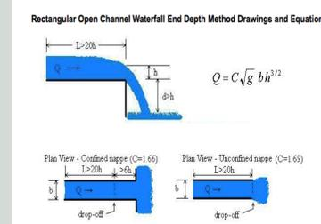
Figure 6. Rectangular Open Channel With Drop Structure (LMNO Engineering, 2015)
