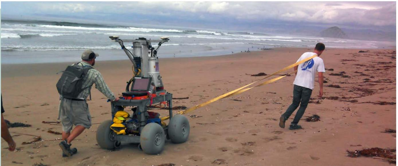
CSU Monterey Bay-CSU Fresno team mapping the Morro Bay sand spit using a terrestrial laser scanner. Image courtesy of Dr. Rikk Kvitek, CSUMB.
