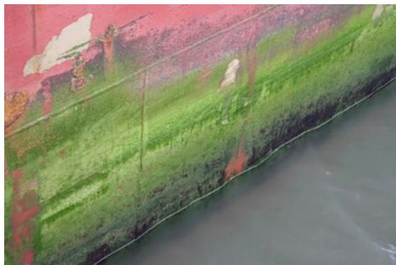
\$800,000 additionally per year. For shipping companies, such as Matson, with 18 ships, that's in the range of \$14,400,000 dollars lost each year, all from a thin layer of slime on the hull of a ship.
