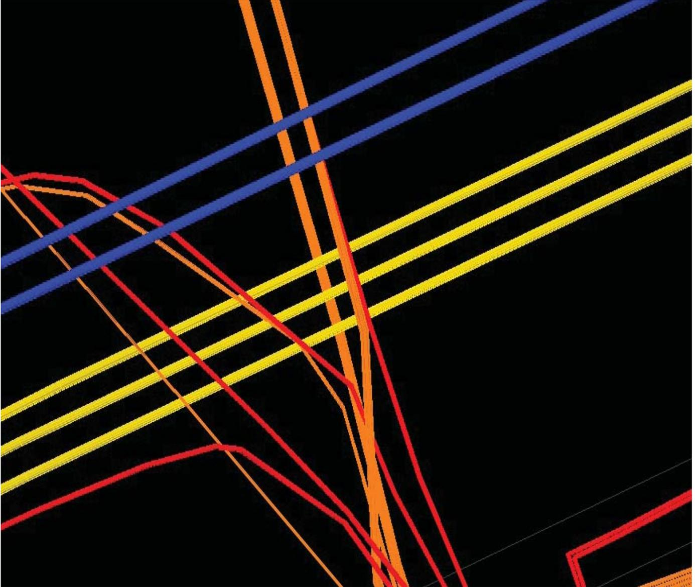
Example 3D Deliverable Civil 3D screen capture. Shows utility lines with relative sizes and position to each other.
