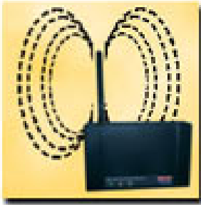
Figure 2 - 8 Omni-Directional Signal Generation The “Doughnut”
